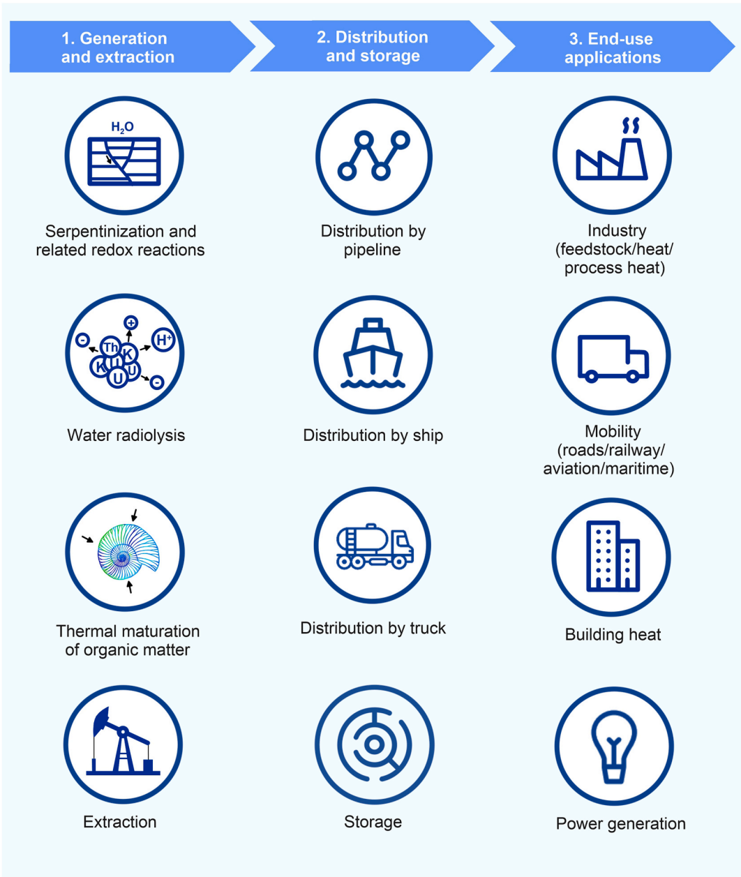
Fig. 1. The role and value chain of natural hydrogen in the energy transition (modified after [8]). The figure illustrates processes capable of generating H 2 in significant quantities and their integration within the broader hydrogen value chain.
