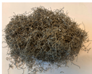
Fig. 4. Recovered smart wire from water-jet delamination route.
