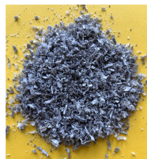
Fig. 9. Recovered polymer sample from water-jet delamination route.
