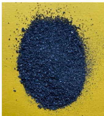
Fig. 6. Recovered silicon powder from water-jet delamination route.
