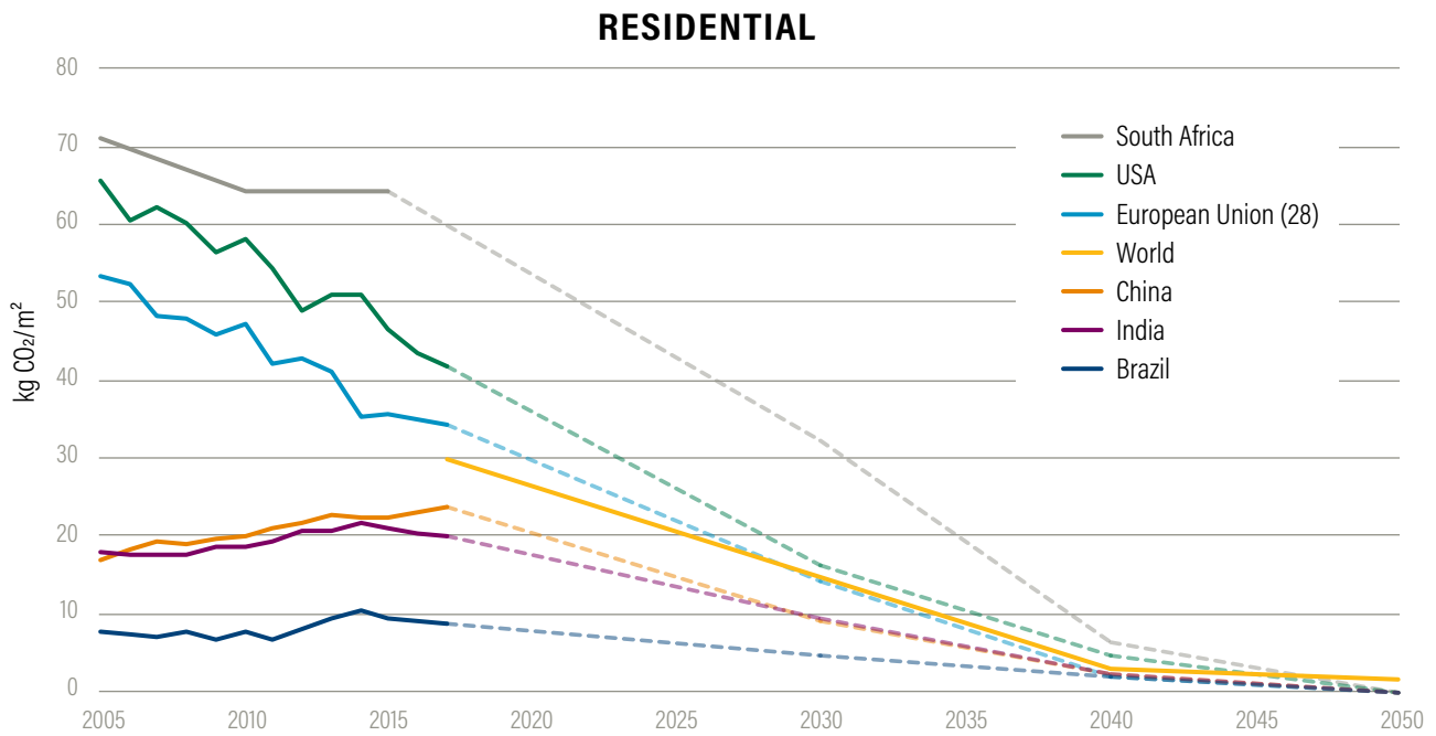
Figure 25 | Historical trends and required decline in the carbon intensity of residential buildings
