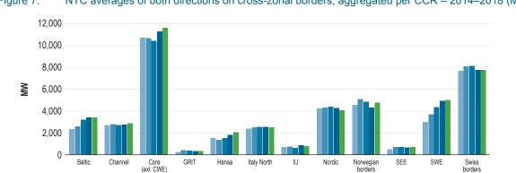
Figure 7: NTC averages of both directions on cross-zonal borders, aggregated per CCR - 2014-2018 (MW)
