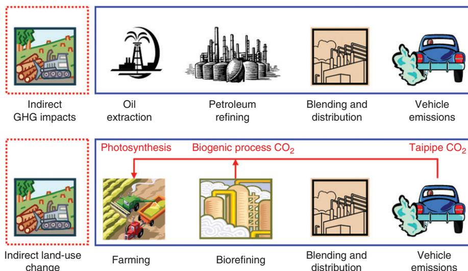
**FIGURE 3** | System boundaries as commonly defined for fuel cycle analysis. (a) Petroleum fuel and (b) biofuel.
