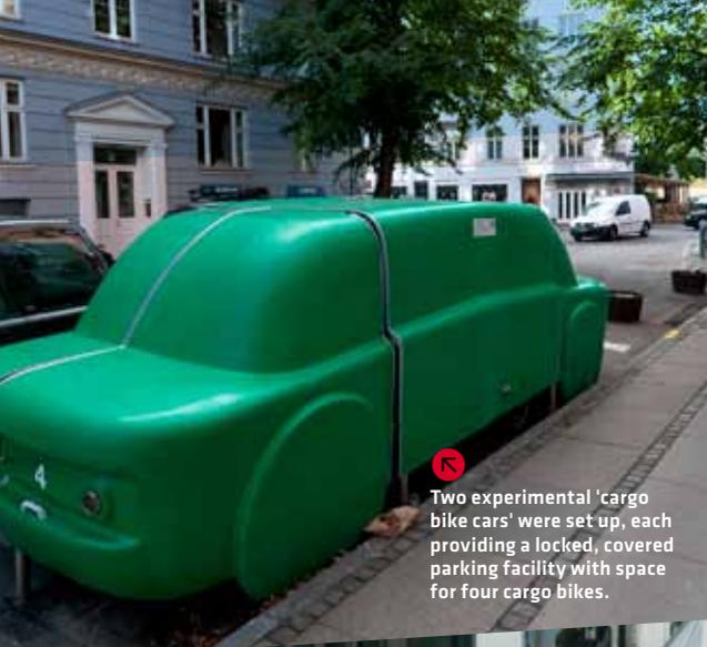
Two experimental 'cargo bike cars' were set up, each providing a locked, covered parking facility with space for four cargo bikes.
