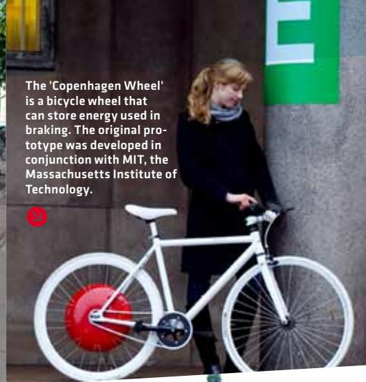
The 'Copenhagen Wheel' is a bicycle wheel that can store energy used in braking. The original prototype was developed in conjunction with MIT, the Massachusetts Institute of Technology.
